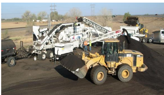
Figure 3. CIR unit set up as CCPR plant (left) and stationary cold mix CCPR plant (right).
