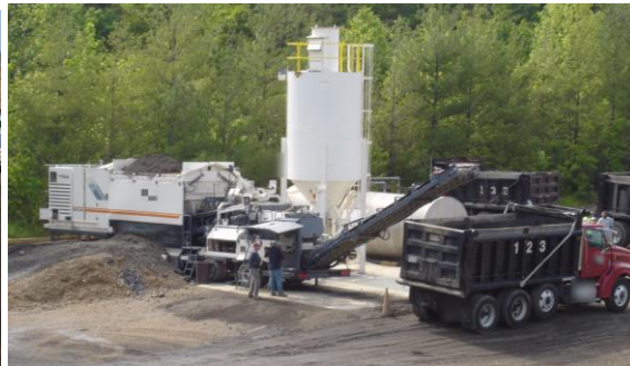
Figure 3. CIR unit set up as CCPR plant (left) and stationary cold mix CCPR plant (right).
