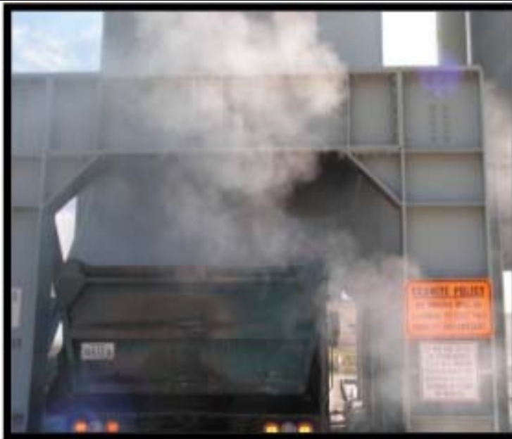
Hot Mix Asphalt at 320°F
