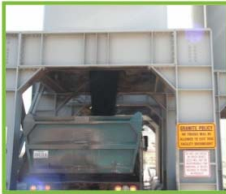
Warm Mix Asphalt at 270°F
