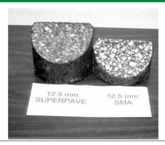
SMA Aggregate Structure. Notice the stone-on-stone contact of the larger aggregate particles.
