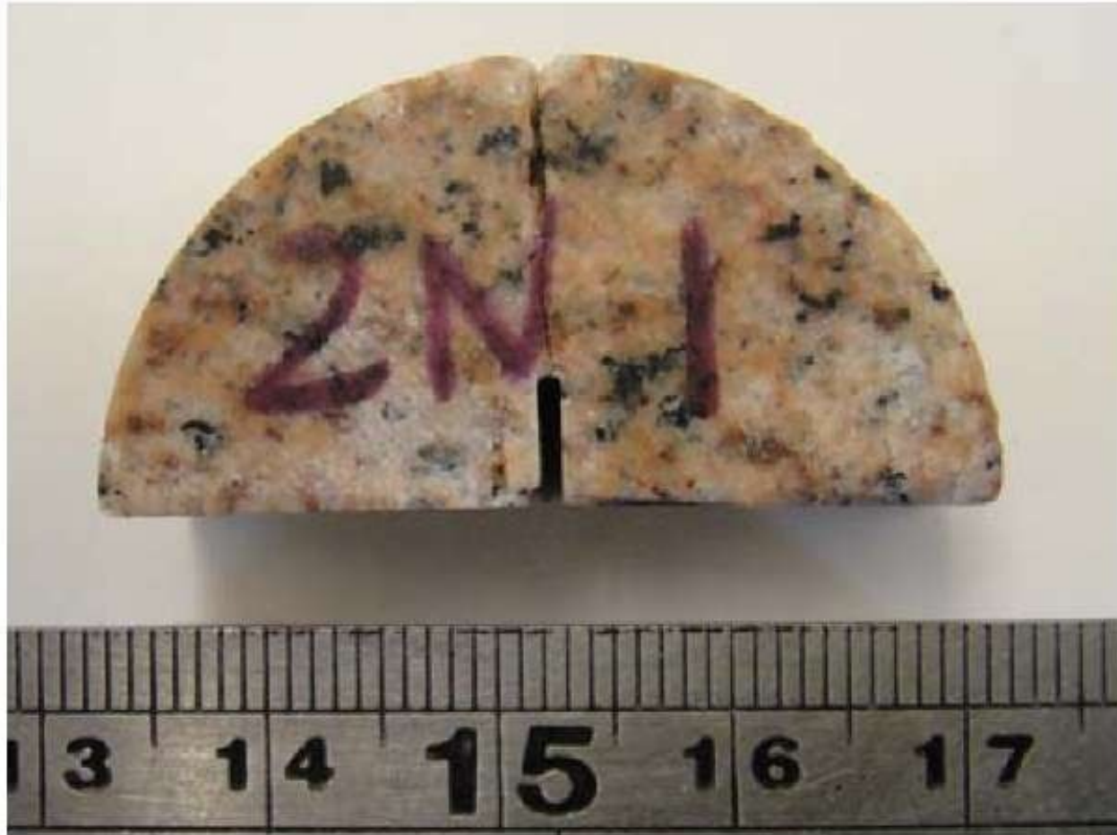
SCB Testing of Granite Rock
